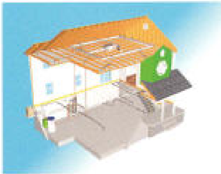
Typical ductwork layouts showing 2 Unico Systems — one located in the attic and one located in the basement.
