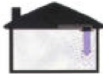
Conventional systems simply dump conditioned air into a room, causing uncomfortable drafts and hot and cold spots.
